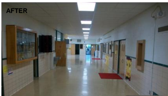
High School Main Hallway: Installed new coiling and replaced incandescent light fixtures with new T8 fluorescent fixtures.
