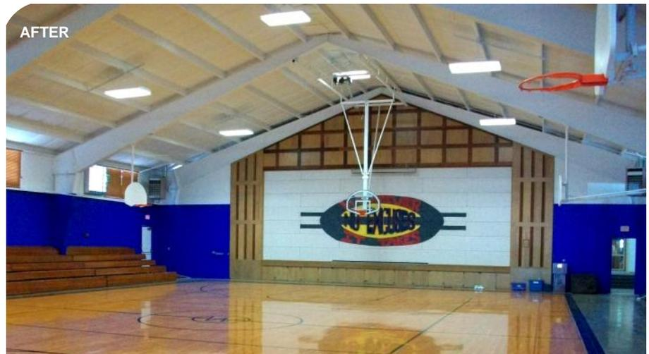
Elementary Gym: Replaced existing metal halide lights with fluorescent fixtures and replaced gym ventilation system.
