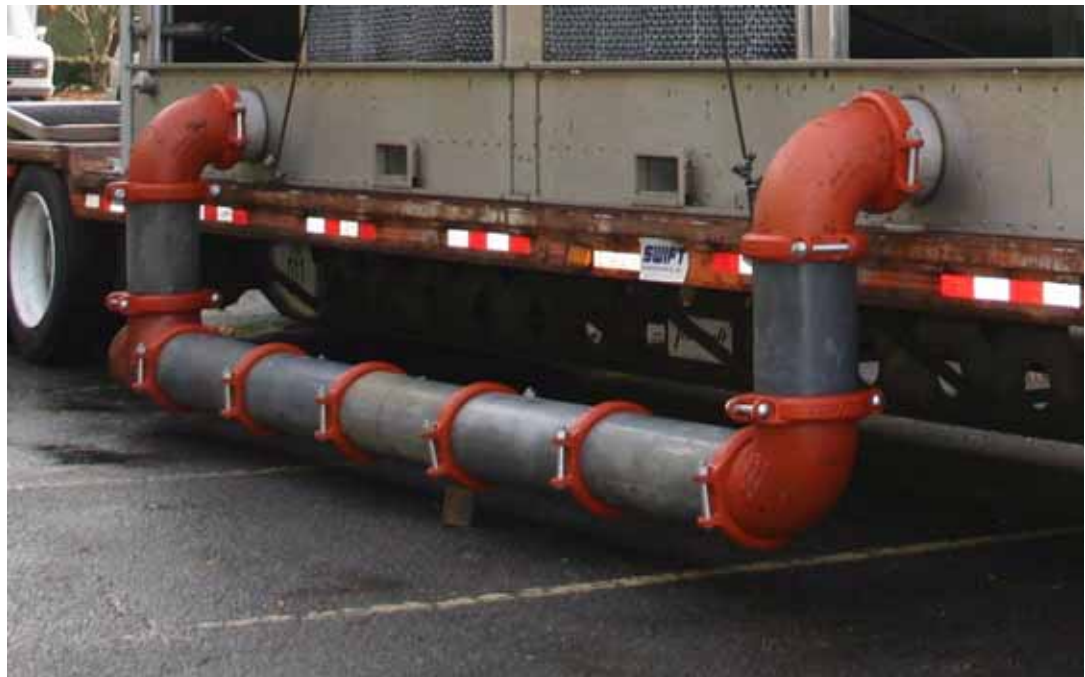
Figure 10. PVC Spool Kit Installation for CSCT00F0AD - AG only
